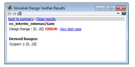
When the software detects an error, the analysis proceeds, but constrains the signal to the tightest intersection of the design range and the derived range, which for the Gain block output in this example is [0..20].
