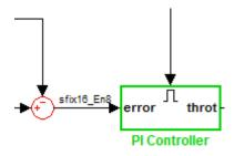
This Sum block can produce an overflow error. The analysis found a test case that can result in a computation where the output of the Sum block exceeds the range [-128..128].
